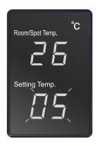
1. When power is on, the set temperature is displayed. Default of set temperature is 5°C.
